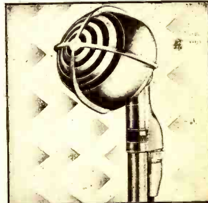
CARDIOID CRYSTAL-LABYRINTH MICROPHONE The Shure "Uniplex" 730-A is a diaphragm-type unit with uni-directional cardioid characteristics (obtained through the addition of an acoustical labyrinth).
