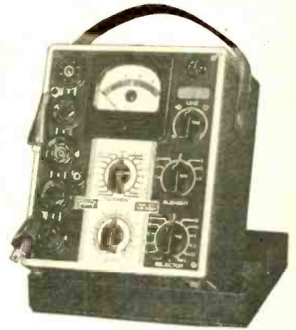
Appearance of the completed "signal substituter". Made by revamping an old radio set, this device demonstrates how a little ingenuity solved problems of economics.
